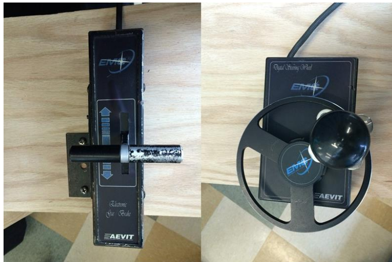
Figure 3 Drive-By-Wire Primary Controls. Left-Gas/Brake Lever. Right-Reduced Effort Steering Wheel
